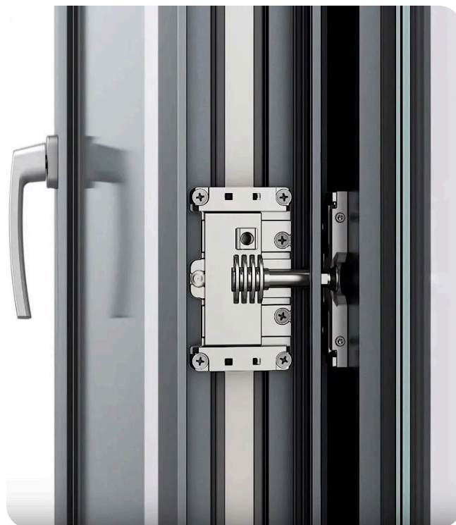
Half a turn. The gear round the panel draws it into the frame, onto the gasket all the way round, and locks at four points.
